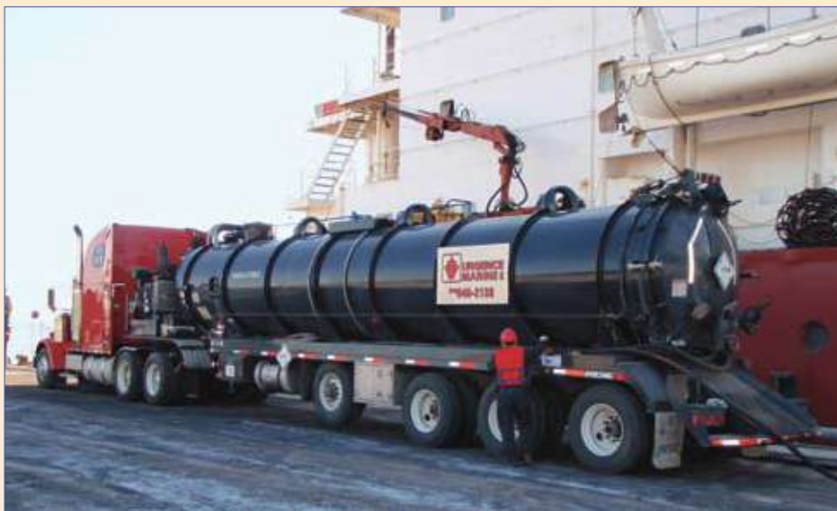
Oily water from vessels is collected by vacuum trucks with capacities of 28 cubic metres.
