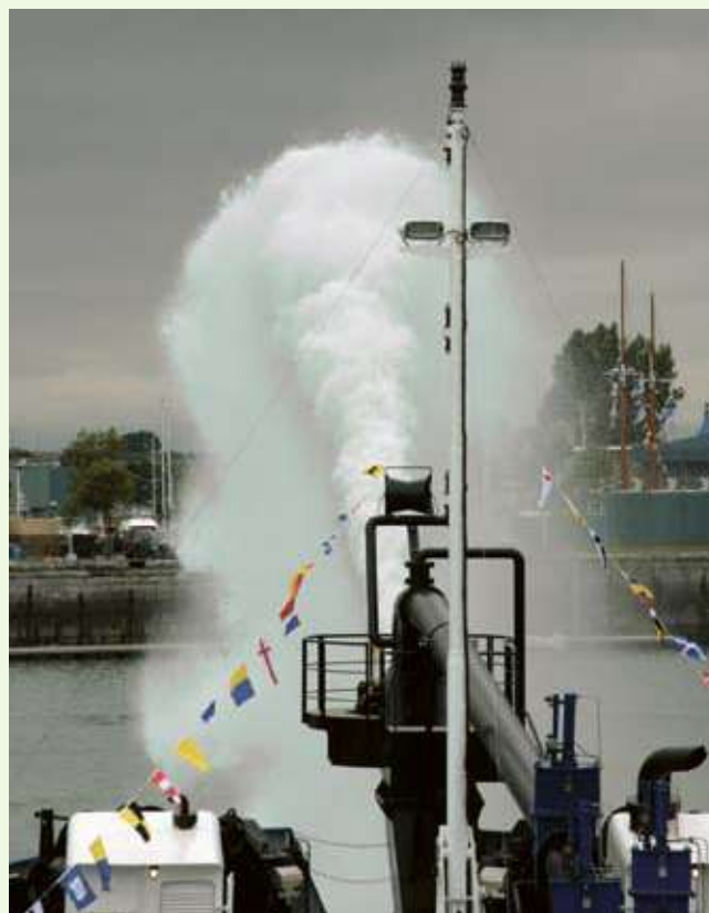
Demonstration of the pump unloading system, which can project its load up to 50 metres away.
