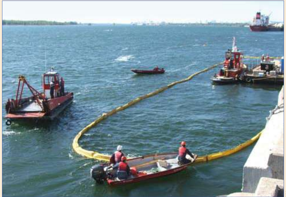
In the event of oil spills, Urgence Marine teams intervene rapidly to contain the spread of the oil slick by installing booms and then proceed with cleaning operations that can also comprise soiled rocks on shore.
